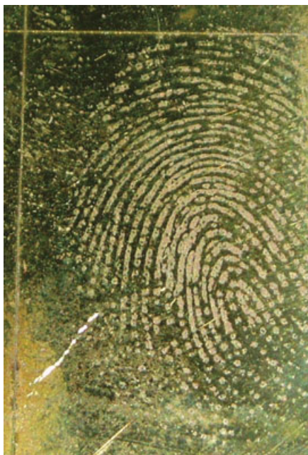
FIG. 7—Photograph of whole fingerprint for sample 5. The horizontal and vertical lines are registration marks used to locate the AFM tip for repetitive examination of the same area of the surface (as in Fig. 10).
