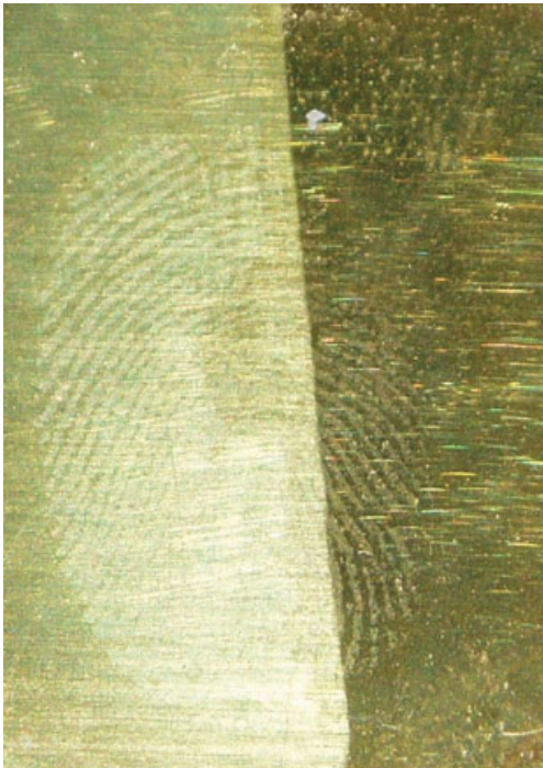
FIG. 1—Photograph of a typical fingerprint on a brass substrate. Prior to deposition of the fingerprint, the left hand side of the substrate was polished (see main text for details); the surface finish of the right hand side is as received.
